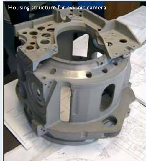
Housing structure for avionic camera
