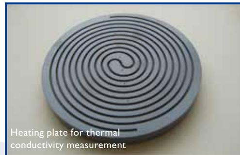
Heating plate for thermal conductivity measurement
